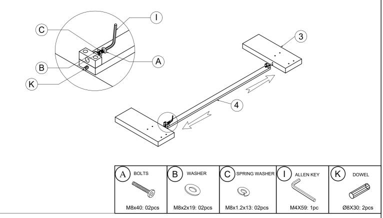
Step 2: Attach the headboard (1) with the legs(3) and bottom stretcher (4) by connecting headboard legs (2), using bolt (A), washer (B), spring washer (C) and using allen key (I)
