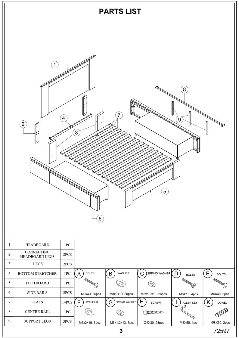
**Step 1: Attach the legs (3) with the bottom stretcher (4)** using bolts (A), washer (B), spring washer (C), dowel (K), and using allen key (I)
